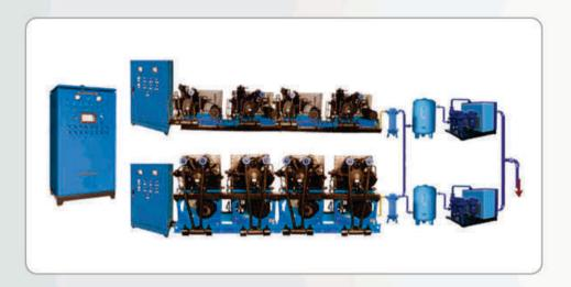
Working principle:Computer-controlled air supply system monitor operation status of blowing machine and demand for high-pressure air, when air demand of blowing machine is low, the air supply system will automatically activate other air compressors, when blowing machine instantly demand a large amount of air, the air supply system will supply the air by making judgment.
